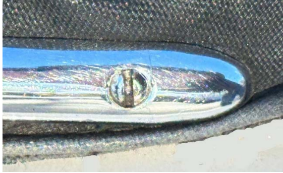
The screws that retain the chrome trim around the bottom of the fabric top are slotted.
