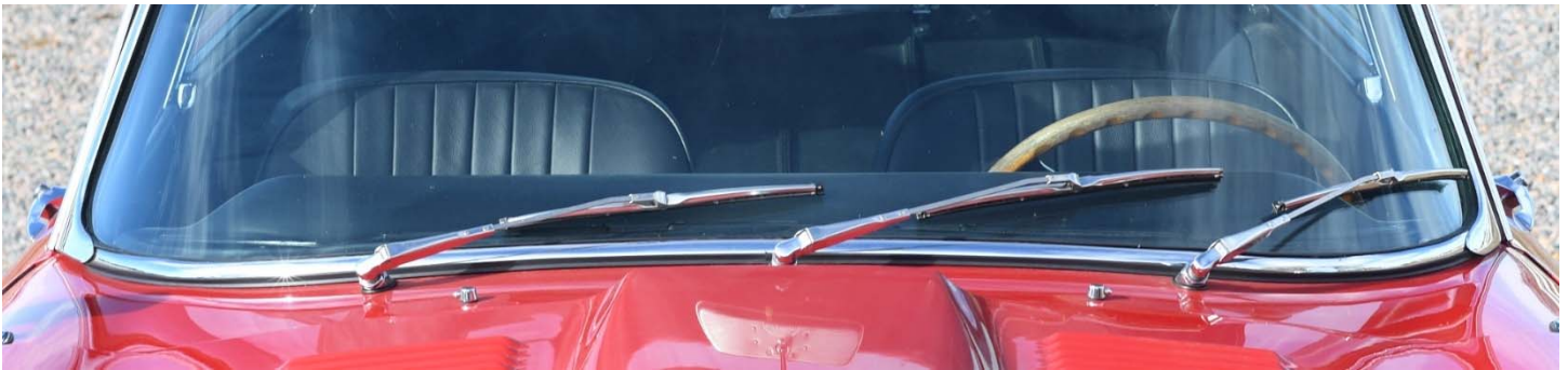
FHC has three Wiper Blades
