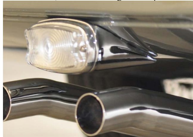
On production cars, the reversing lamp is located above the twin exhaust pipes.
