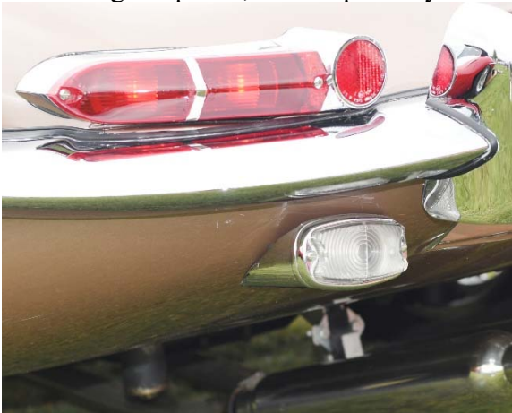
On very early E-Types, the reversing lamp is located near the left bumper over-rider.
