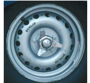
D-Type & Some E-Type Race Car Wheel, Round Holes Courtesy Terry Larson
