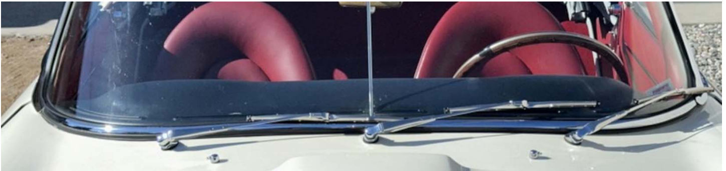
The wiper blades are shorter on the OTS
