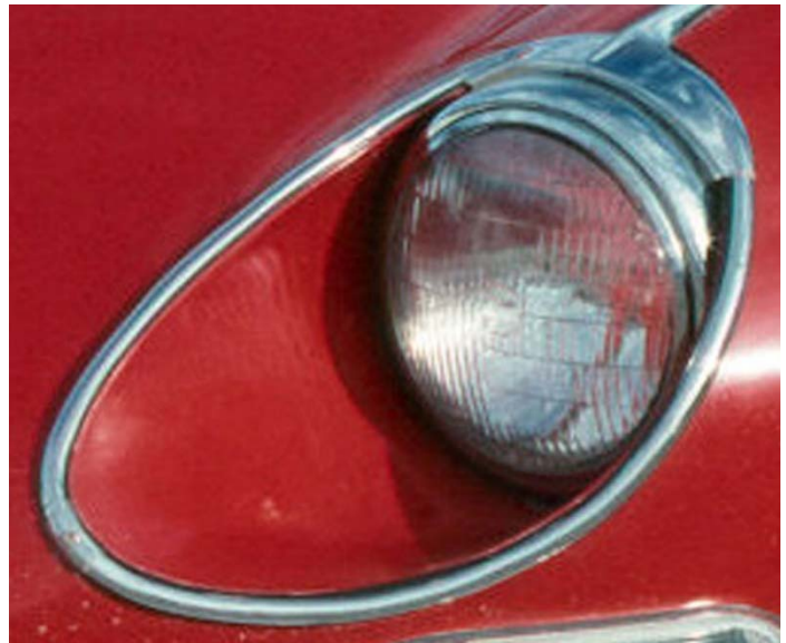
Uncovered Headlamps and Body Colored Headlamp Buckets
