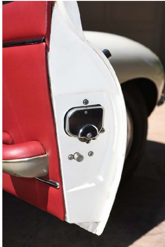
B-Post Shut Face and Latching Mechanism
