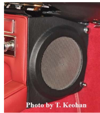
4.2L with satin finished grill and black grill surround that is part of the black vinyl covered console side panel.
