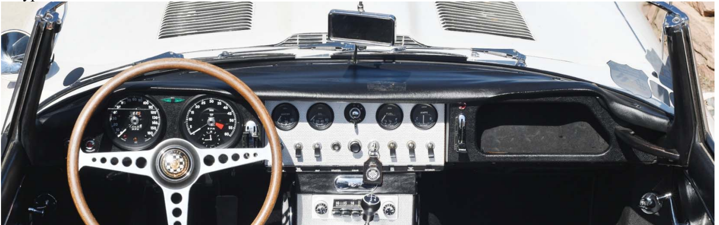
3.8L Left and right-side portions of the dash are black vinyl. Center dash is dot pattern aluminum. Early car with a flat vinyl dash top.
