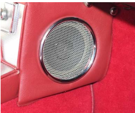
3.8L has satin finished grill and chrome surround mounted on the side of the upholstery-colored leather covered console panel
