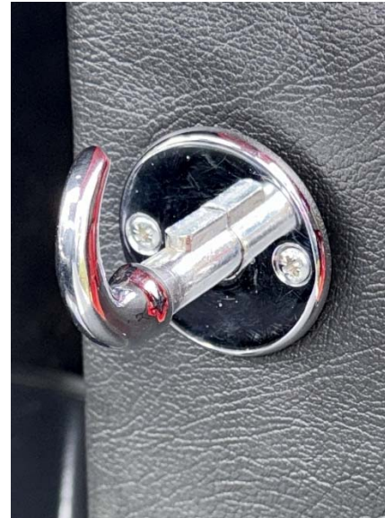
Bonnet “J” Release Handle and escutcheon, mounted with either Phillips Head or Pozidriv Screws, on 4.2L car and the “J” Hook is at the top when open.
