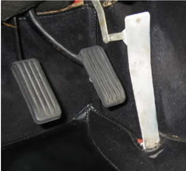
3.8L Pedals, brake pedals are flat with vertical ribs. The accelerator pedal has a slight bend near the middle.
