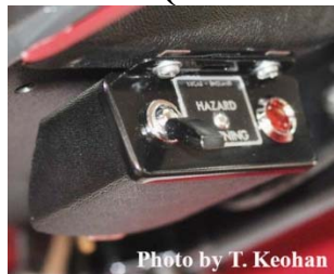
A cover plate is added to the back of the Warning Device; however, no exact chassis number is given.
