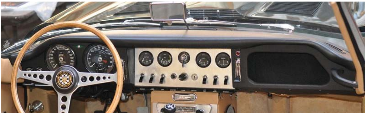
3.8L Left and right-side portions of the dash are black vinyl. Thicker dash top. Cross-hatched instrument panel.
