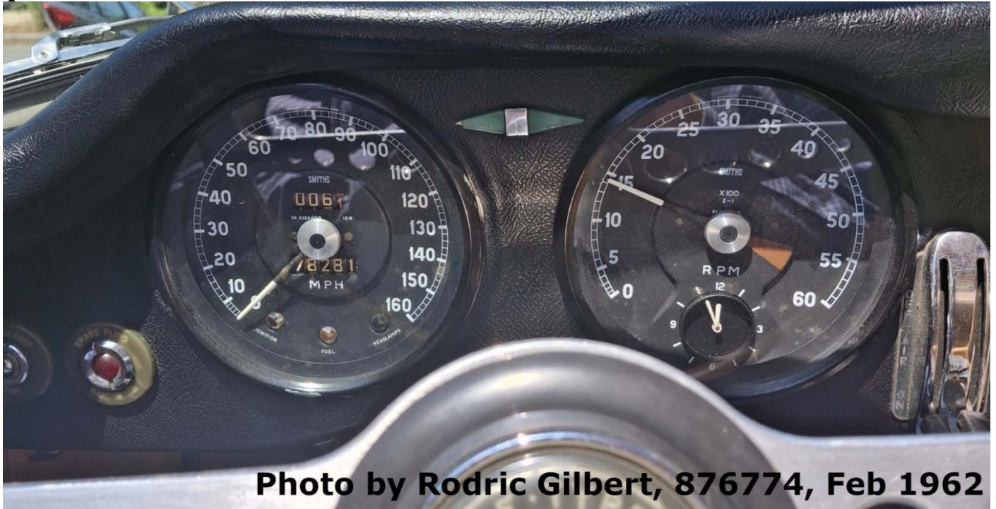
3.8L Speedometer and 5500 to 6000 RPM Tachometer
