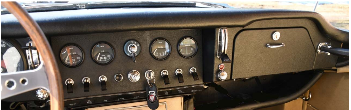
4.2L Left and right-side portions of the dash and instrument panel are black vinyl. Locking glove box (1E.77148 shown here)
