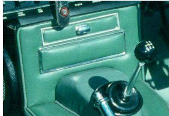
When the radio was not supplied, the upholstery colored "Radio Delete" panel was installed
