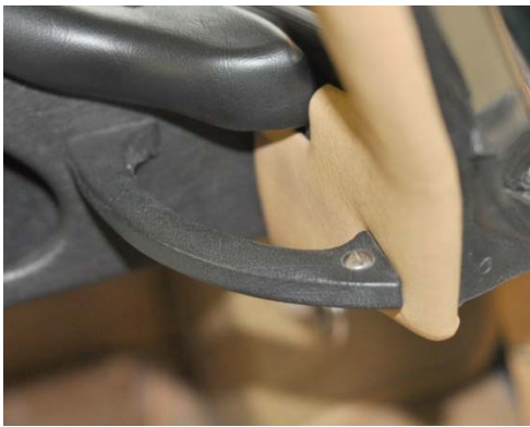
3.8L Grab Handle is fastened from the back to the dash and fastened to the windshield pillar by a slot head screw.
