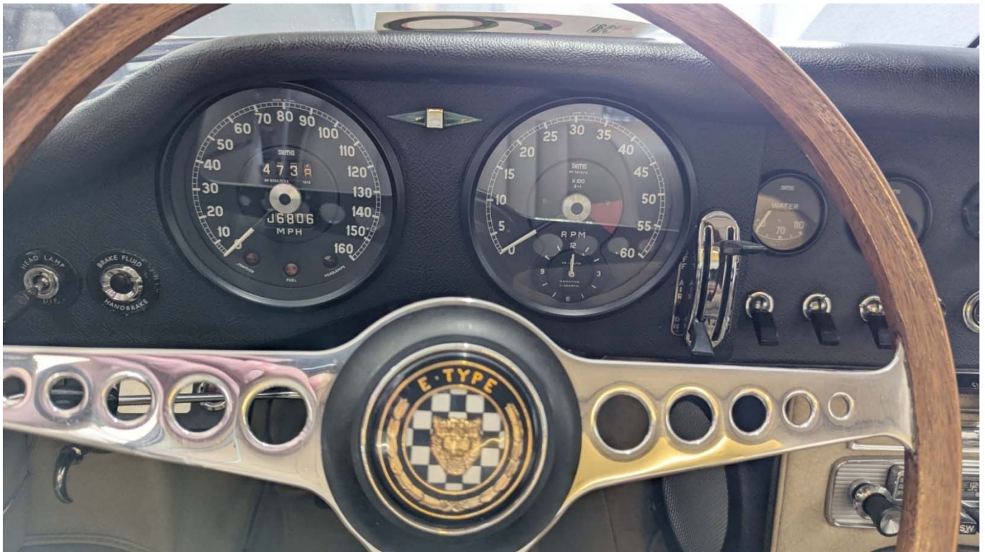
4.2L Speedometer and 5000 to 5800 RPM Tachometer
