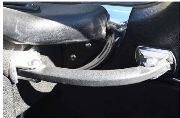
4.2L Grab Handle is fastened to the dash and the windshield pillar via chrome mounts and held in place by chrome, dome head fasteners.
