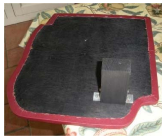
Second style of back of toe-board with a block support
