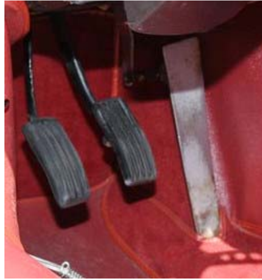
4.2L brake pedals are curved with vertical ribs. The accelerator pedal is straight.
