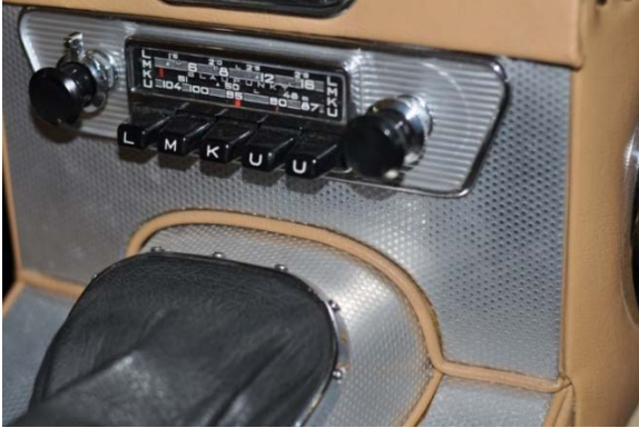
The 3.8L Radio bezel, for the aluminum Dot or Cross-Hatched pattern, has a horizontal pattern and the shape is trapezoid.
