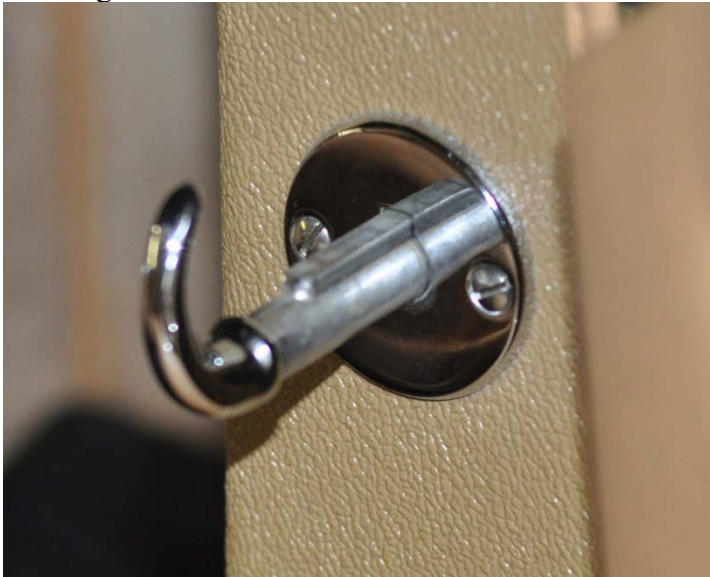
Bonnet “J” Release Handle and escutcheon, mounted with Slotted Screws on 3.8L car and the “J” Hook is at the top when open.
