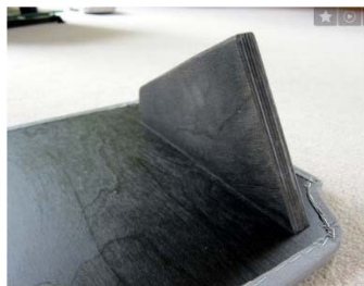
First style of back of toe-board with a triangular support
