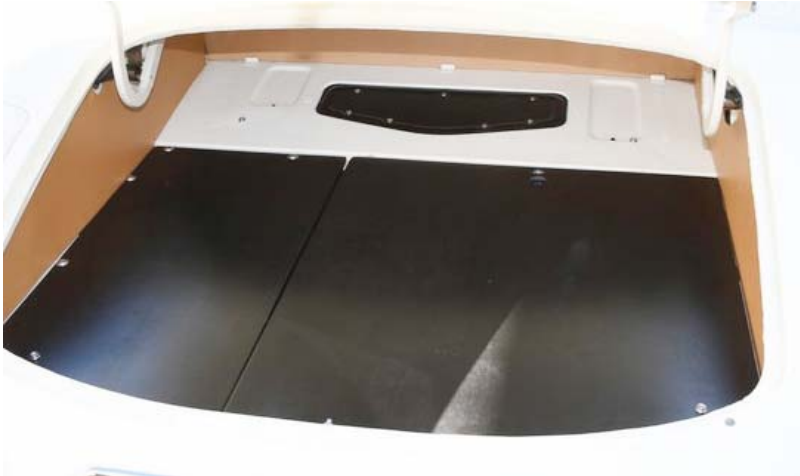
The plywood panels covering the gas tank and spare tire are painted a semi-gloss black
