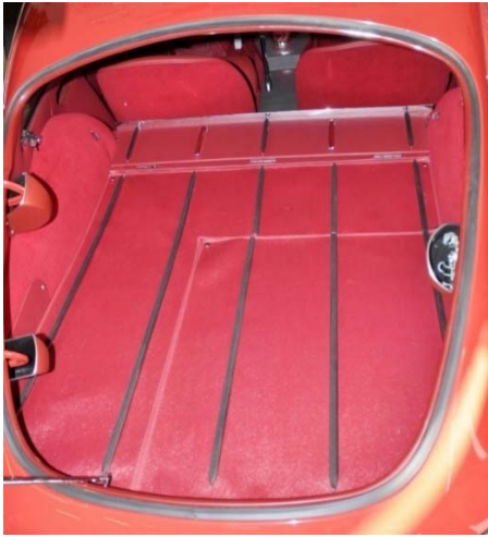
3.8L Fixed Head Coupe, Moquette Trim. Early 3.8L FHCs have a two-piece boot mat.
