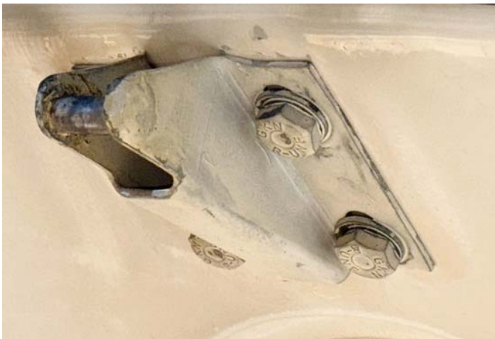
The boot lid latch and bolts are cadmium plated Note: Show here is unrestored 875950
