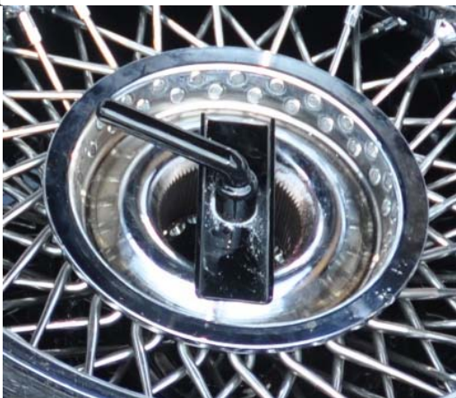
The Spare Wheel and Tire retainer or hold down has a black handle and hold down plate. The threaded shaft is cadmium plated.
