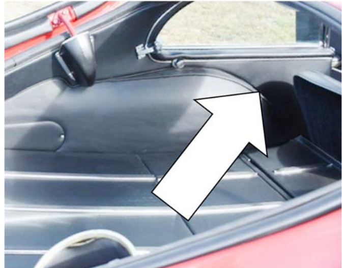
Vinyl covered wheel arches and pocket deleted from the side casing panel.
