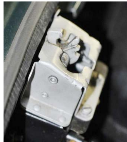
OTS Locking Assembly and cheese head screws are cadmium plated.
