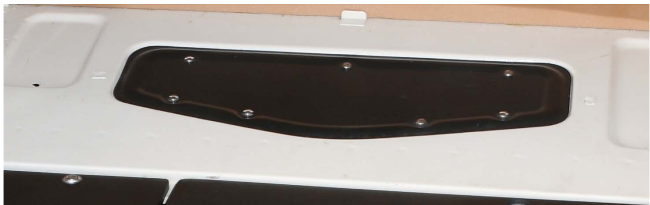
The differential access panel is semi-gloss black, held in place by cadmium plated slotted screws.
