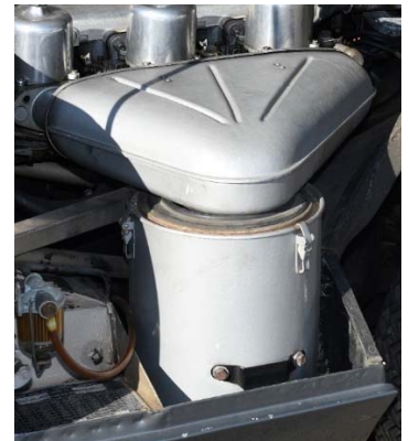
Some late 3.8L and most 4.2L filter canisters have the three recesses or groves and are the same Hammeritone gray as the air plenum.
