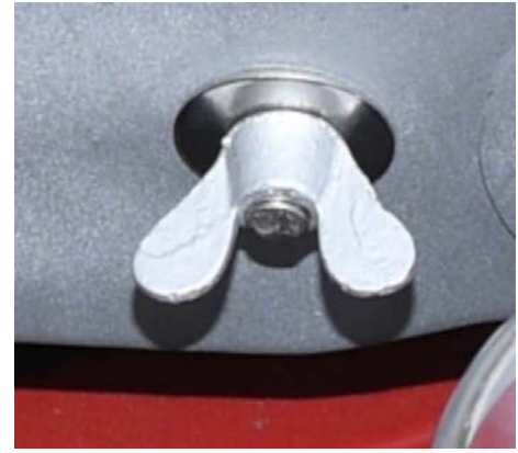
Large Eared wing nuts holding the Trumpets to air plenum
