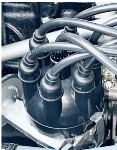
3.8L & 4.2L with Rubber Boots Covering Plastic Nuts
