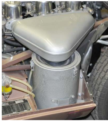
Most 3.8L filter canisters are the same gray as the air plenum.
