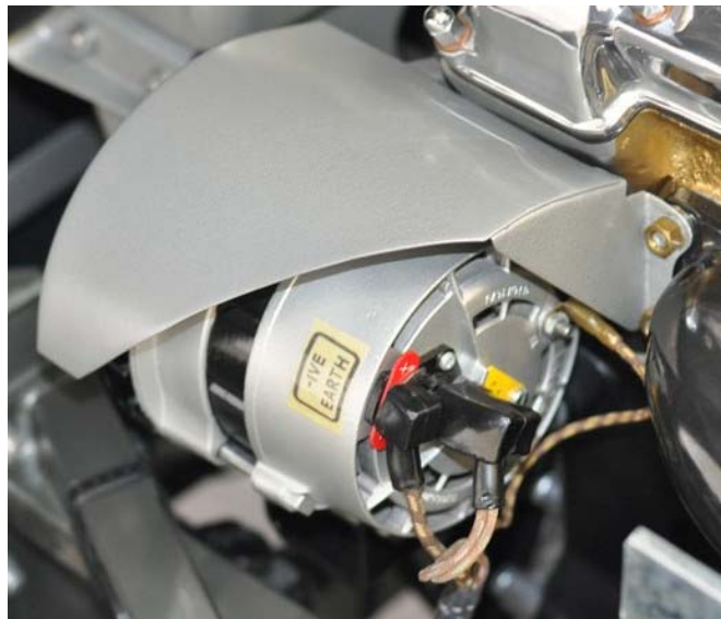
4.2L Alternator with a Hammertone heat shield fitted at engine number 7E6333.
