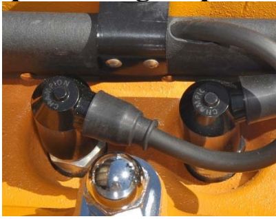
Black spark plug cap with a dot in the center and non-painted "Champion" lettering in a circular pattern on top, used on very early E-Types.
