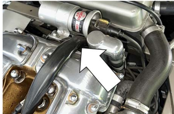
4.2L Spark Plug wire routing is encased in a PVC sleeve and routes behind the coil.
