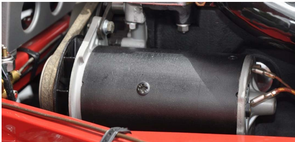
The 3.8L generator housing is flat black with aluminum end plates.
