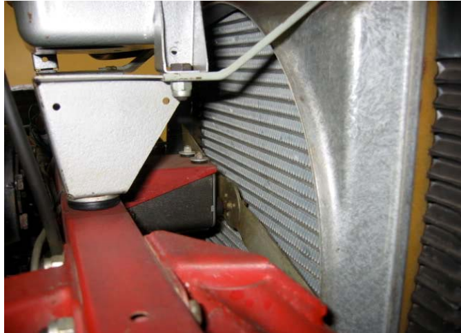
October 1962, SB D.6: The fan motor relay, mounted on the right side of the gray header tank support, is discontinued.
