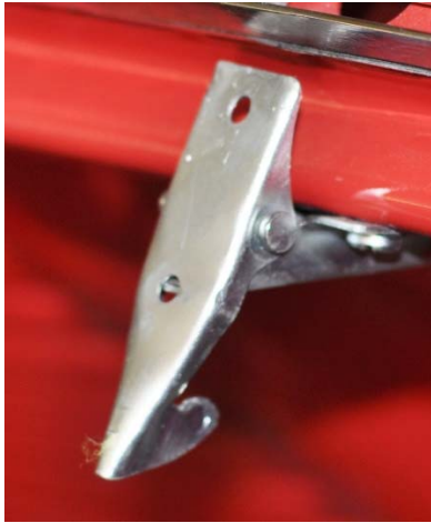
Bonnet Safety/Receiver Catch Bonnet catch and latch are cadmium plated.
