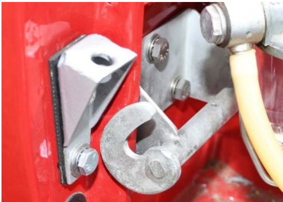
Cadmium plated Bonnet Stop & Lock Assembly
