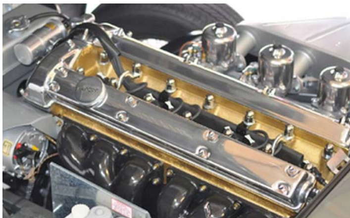
4.2L, Black spark plug conduit routed through PVC shield from front of cylinder head.
