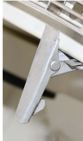
Bonnet Safety/Receiver Catch Bonnet catch and latch are cadmium plated.
