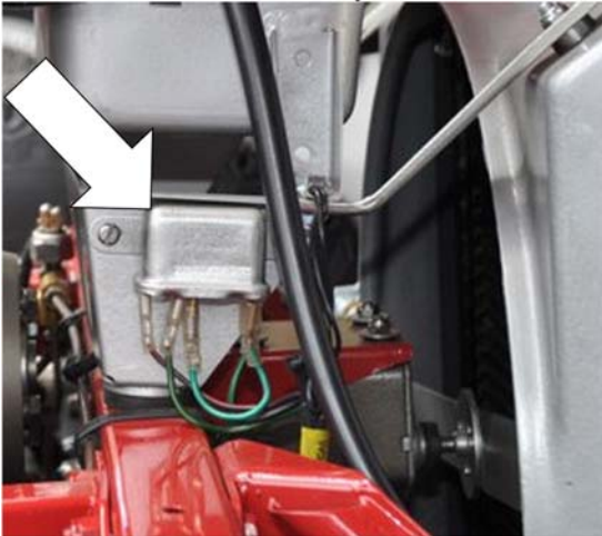
October 1962, SB D.6: The fan motor relay, mounted on the right side of the gray header tank support, is discontinued.
