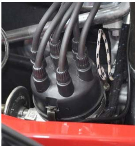
3.8L & 4.2L with Plastic Nuts, but missing Rubber Boots
