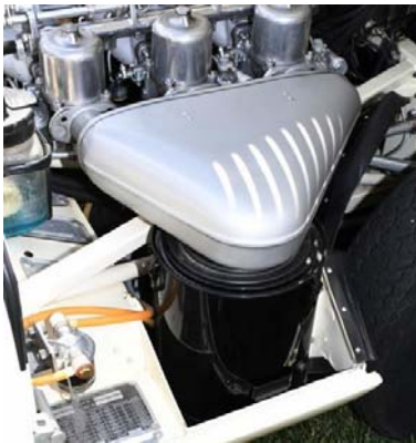
The 3.8L has a smooth Air Plenum. Some have black filter canisters.
