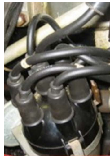
The change from threaded spark plug wire nuts to push-in spark plug wire plugs was around March 1968.
