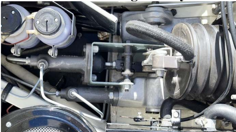
3.8L brake and clutch master cylinders are natural cast aluminum. Brake bellows is black.
