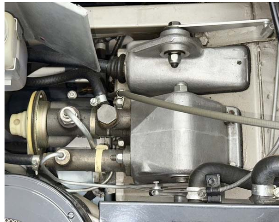
4.2L brake and clutch master cylinders are natural cast aluminum. The brake booster, located on the lower portion of the engine side of the bulkhead below master/clutch assembly, is black.
