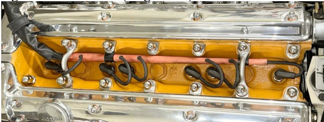
Early 3.8L E-Types have red fiberboard spark plug conduits.
