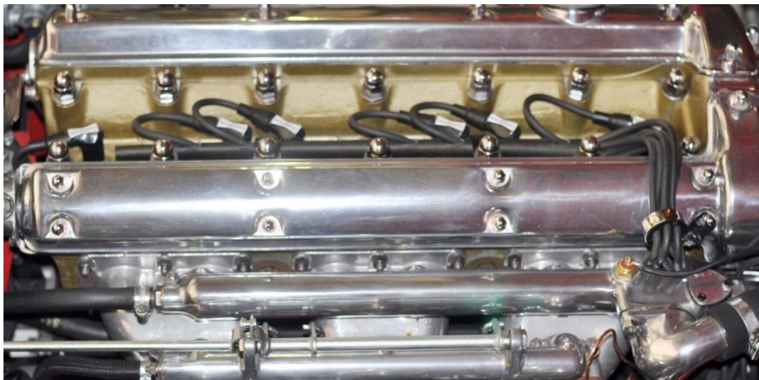
886838, 3.8L E-Types have a black fiberboard spark plug conduit. The spark plug wires are routed up from the distributor, through a round ignition wire separator with the chrome bracket.
