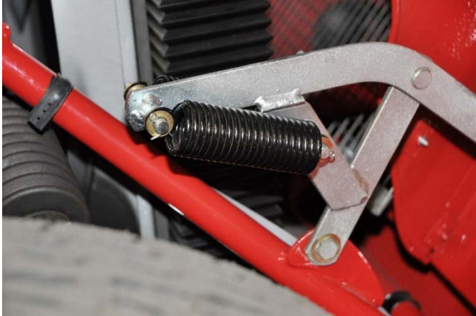
Bonnet Compensator, cadmium plated, Bonnet Springs, gloss black
