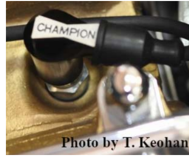
Black spark plug cap with the white painted "Champion" "Bow Tie" on top of the cap used on most 3.8L and 4.2L E-Types.
